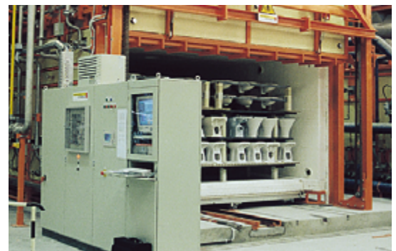
Intermittent shuttle kiln in the ceramics industry
